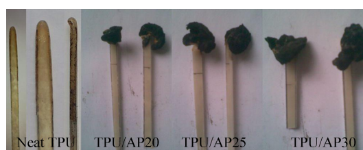
Fig. 1 Digital photos of the residual chars for neat TPU and TPU/AP systems after the LOI tests
